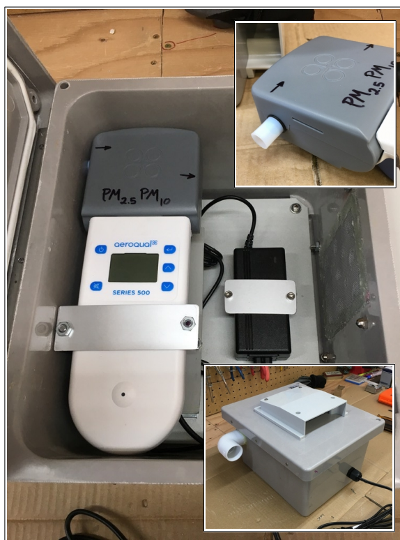
Figure 2.4: Custom enclosure built by Inversion Labs for the Aeroqual S500 PM_{2.5}/PM_{10} monitor. Sampling of ambient air through the enclosure wall was enabled with a 1.5 cm length of PTFE non-reactive tubing.
